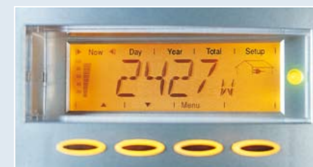
The Fronius Personal Display shows current data from up to 15 inverters.
